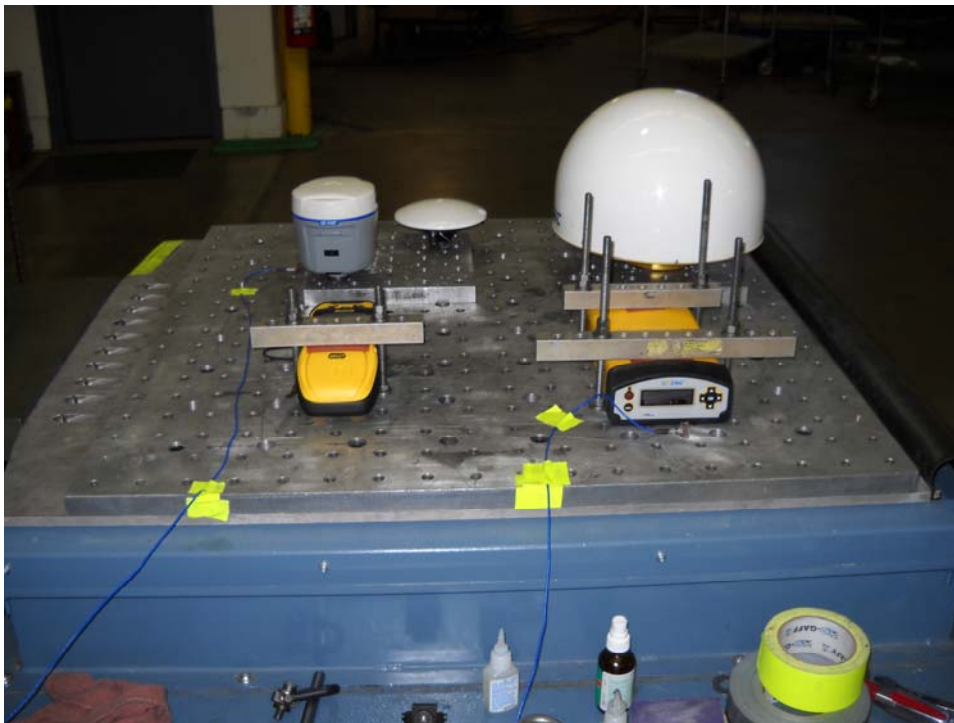
Photograph 4-8: Test units secured to the slip plate and ready for testing in the transverse axis. The control accelerometers are visible, cemented to the slip plate. Applied motion is left-to-right as this photograph is viewed.
