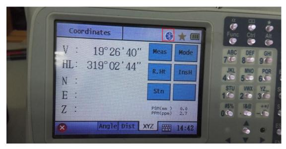
4. In measurement screen when you see bluetooth Symbol, it means Bluetooth is turned on.
